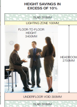
Floor Designed with Underfloor Air Distribution System
