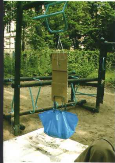
Basic load test of bolted connection between sheets of honeycomb cardboard. The local playground was used as a test site.
