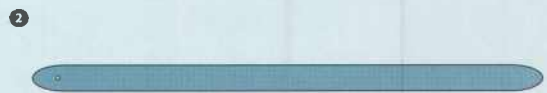
The tubes are sealed at the ends and valves added for inflation. At this stage a partially inflated tube will adopt a straight condition.
