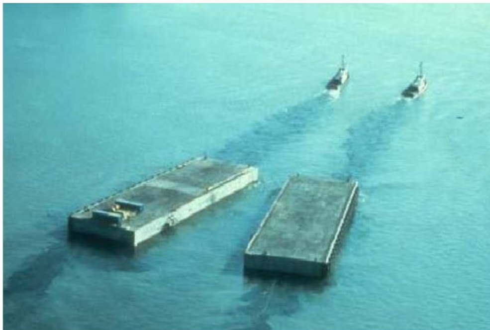
31. Towing Concrete Pontoons
