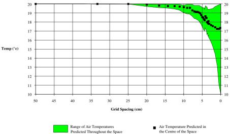
It can be seen that the predicted air temperature in the centre of the space decreased by almost 2.75°c as the grid spacing became smaller. This was as a result of *Flovent* being more able to simulate the fast moving down draft close to the cold surface, resulting in increased convection heat transfer at that surface.
