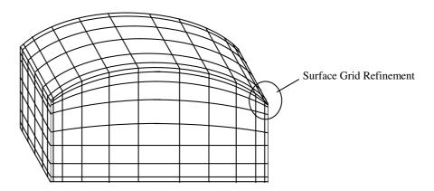
Flovent was unable to generate such a BFC grid. Some existing CFD codes are based on BFC grids (*Phoenics*<sup>[27]</sup>) or even unstructured grids (*Fluent*<sup>[28]</sup>), but in order to accommodate some of the other developments suggested in this section, it seems likely that a purpose written thermal model may have to be developed.
