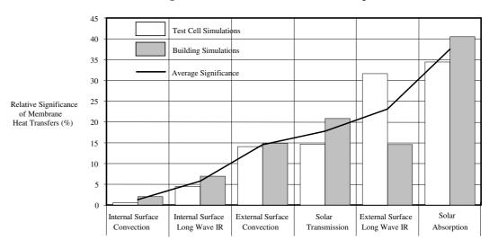
Figure 10:2.2c Diagram to show the Relative Significance of the Membrane Heat Transfers
