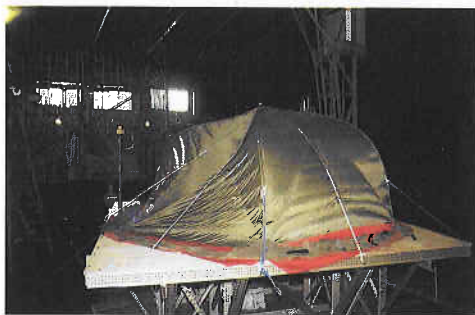
Fig 12.1 Prototype under test in the 24' diameter open jet wind tunnel at Farnborough
