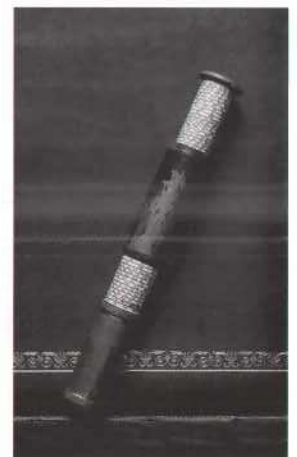
Ted's cylindrical slide rule
