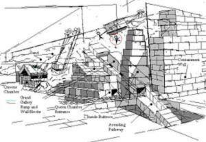
Here is sorther distriction showing how the entrance to both the Orand Osloy and the shaft boding to the Queens chamber would come using play. Multiple construction areas would be going on at the same time so that corrections can be made while they are still accossible.
