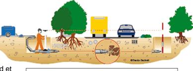
Image: Trenchless technology taking place as to not disturb traffic <u>http://www.hms-it.co.uk/trenchless\_technology.htm</u>
