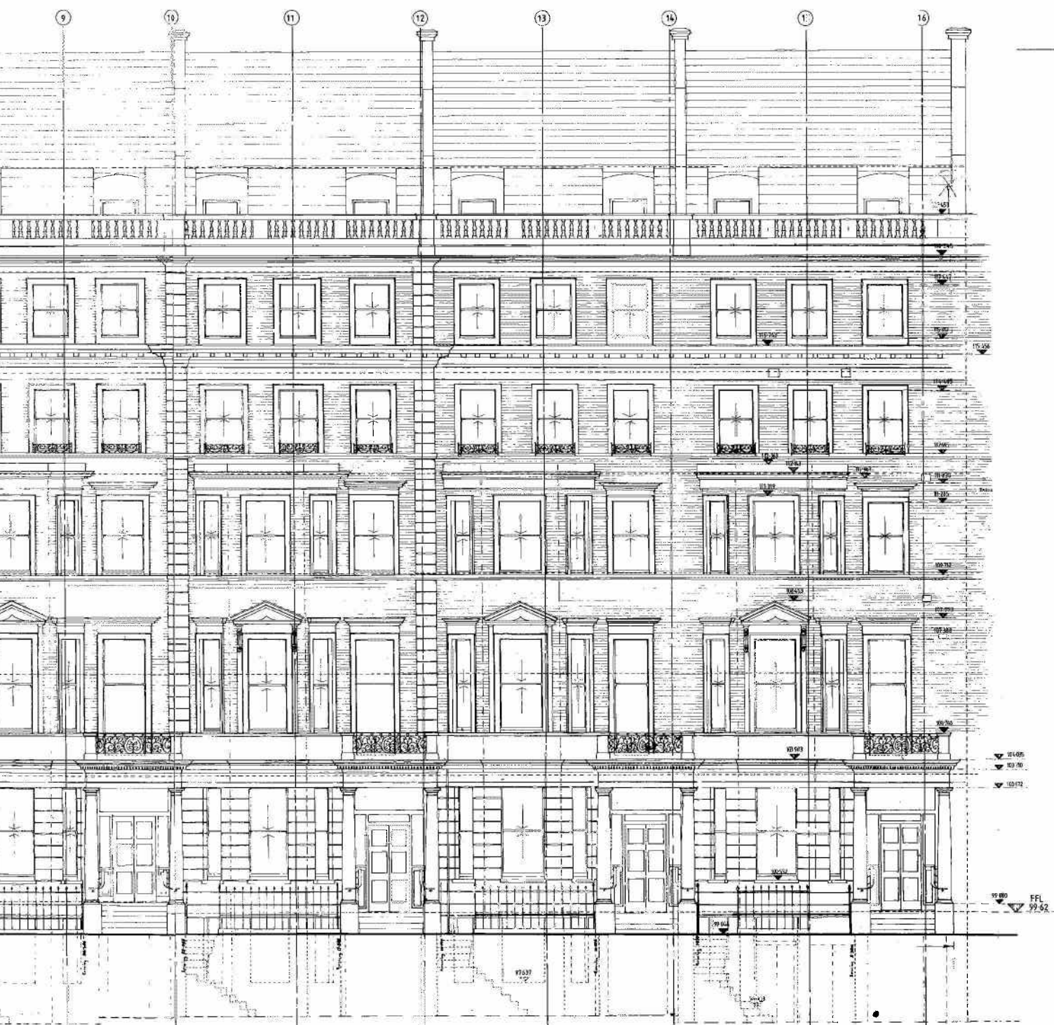
Fig 7.2 Elevation of terraces, showing new floor levels
